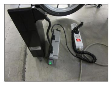
4) Charging in progress: the fans of the battery charger are running, the green lights on the percentage of charge already present in the battery light up and the remaining green lights start flashing; as the battery charges, the lights of the relative percentage of charge reached remain on steady.
