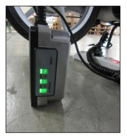
If the battery connected to the charger is damaged, the charger's fans are active and the green lights are on and off, as in the picture below.
