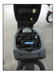
2) Remove and disconnect the charger, then lift the battery slightly, disconnect it from the connection cable and remove it from the battery compartment.
