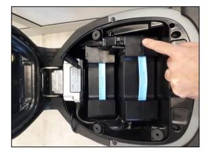
3) Battery B (towards the front of the vehicle) connected:
